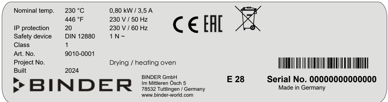
Figure 2: Type plate (example: E 28 regular chamber)
