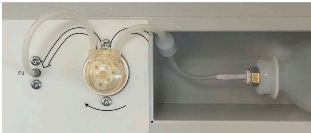
Figure 21: Installation of the water supply via prefilled water bottle, assembled
