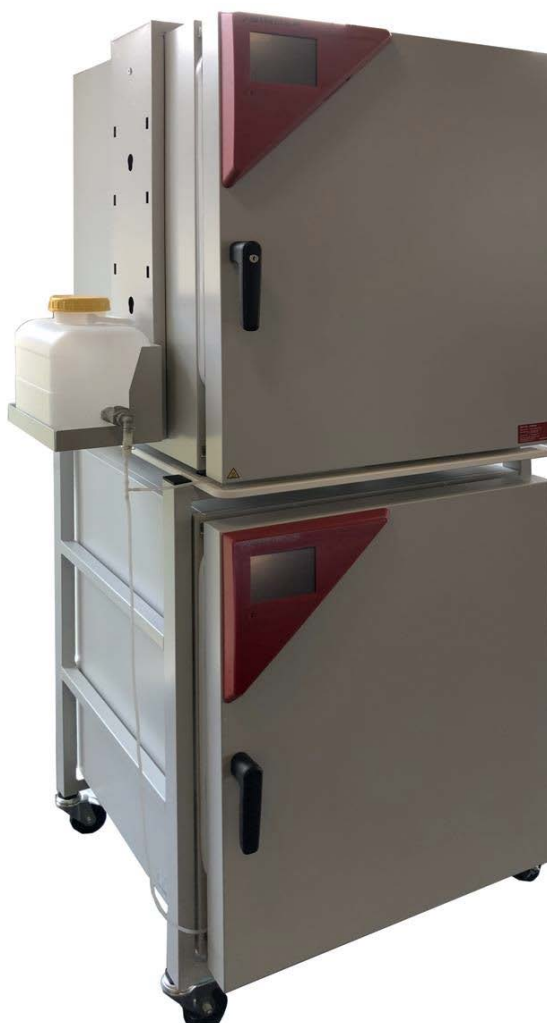
Figure 24: Two CBF / CBF-UL incubators with installed water supply via freshwater can (accessory)
