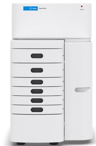
The Femto Pulse system uses a pulsed field power supply along with quantitative and qualitative kits to automate the separation of genomic DNA as large as 165,000 bp, DNA smears, DNA fragments and RNA.
