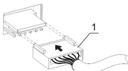
**Figure 1. Thermoblock connection**
